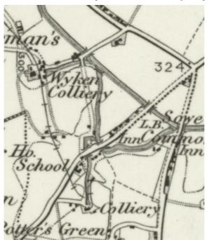
detailed more 1913 Ordnance Survey indicates that all canals in the area were still navigable together with colliery railways, even clearly showing redundant earthworks of the original Oxford Canal route paralleling the Coventry to its original junction at Longford Bridge on Bedworth Road. Wyken Old Pit has closed but clearly from census returns, other collieries remain very shortly busv. However afterwards in 1915 remaining colliery in Wyken closed followed ten years later by Craven colliery.
